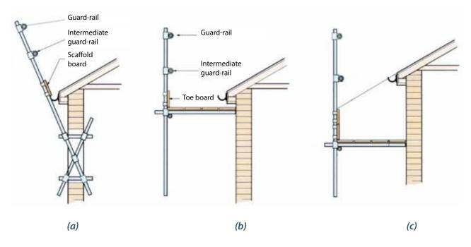
Figure 8.8: Typical sloping roof edge protection. Barriers shown in (a) can be useful where space is limited but they are not capable of sustaining loads as large as (b) and (c), which also provide a working platform.
