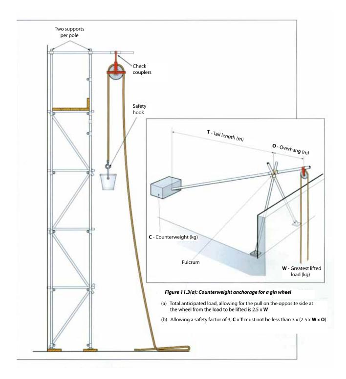
Figure 11.3: Properly erected gin wheel
