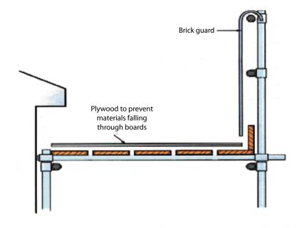
Figure 11.6: Suitable protections where the public could be at risk from falling objects or materials.
