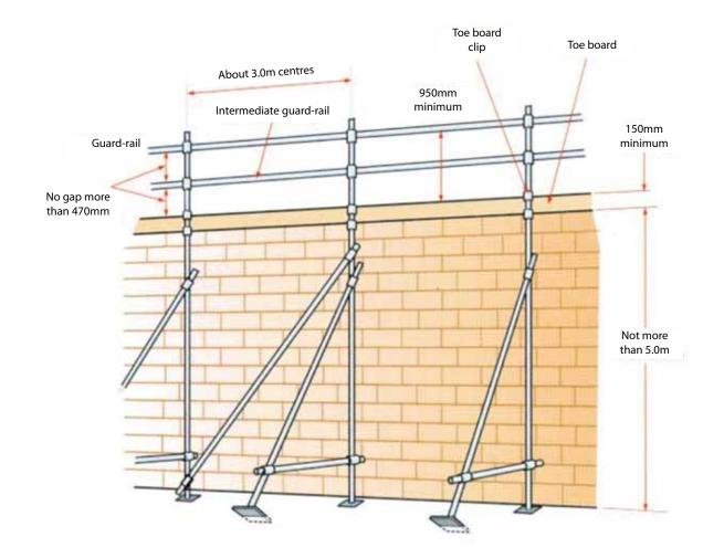
Figure 8.6: Flat roof edge protection supported at ground level. Ground level supports allow work at roof level without obstruction.
