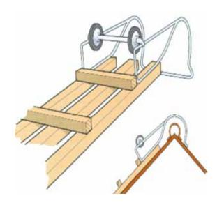
Figure 11.2 Roof ladder. The ridge iron should be large enough to clear the ridge tile.
