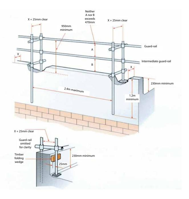
Figure 8.7: Flat roof edge protection supported on the roof edge upstand. The roof upstand must have adequate strength.
