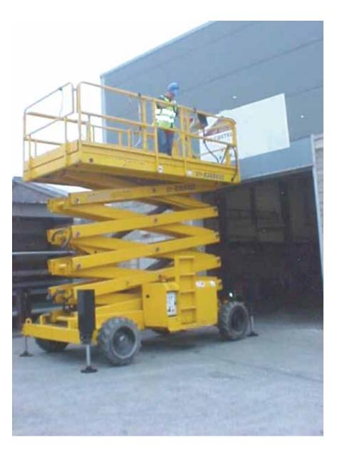
Figure 13.2: Simple mobile access used for short term work at parapet level.
