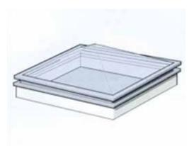
Figure 4.7: Typical out of plane rooflight
